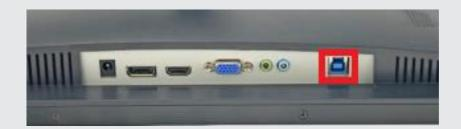
Using the USB-A connection, please connect this directly to your PC/Terminal. Your Windows PC/Terminal will automatically detect the new hardware and you should find that applications now detect your Webcam and Mic.
